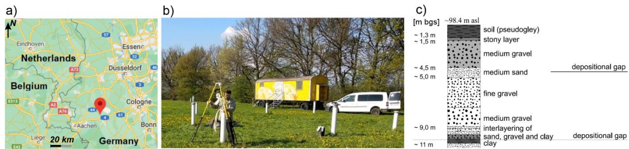
Figure 1: Krauthausen test site. a) Location of the test site in western Germany (red dot). b) Image collected during GPR crosshole acquisition. c) Generalized cross-section of the investigated aquifer at the Krauthausen test site (modified from Englert, 2003).
