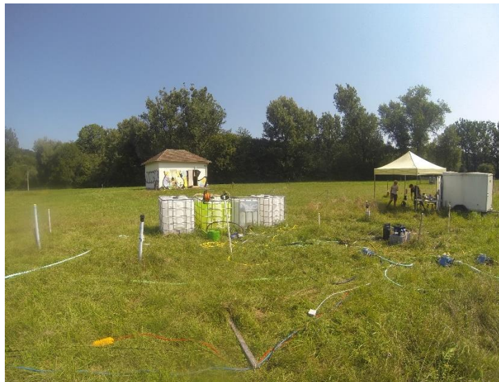
Figure 13. Impressions from the field site during the tracer test. Four tracer mixing tanks were prepared for tracer injection (green = fluorescein).
